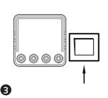
After the wiring of switch module is done, press the traditional switch to turn ON/OFF cycle for 5 times (keep time interval not too short) until the indicator light flash for pairing mode.
