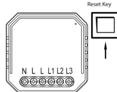
After the wiring of switch module is done, press the traditional switch to turn ON/OFF cycle for 5 times (keep time interval not too short) or press the reset key for about 10s until the indicator light on the module flash quickly for pairing mode, if the indicator light flash slowly, pls repeat the above procedures.
