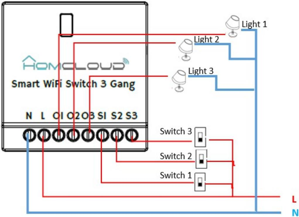
4) Wiring diagram of **single pole dual control switches** as Traveler system
