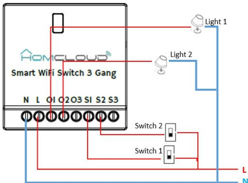
Remark: The connection of two-way switch is only valid in the above connection mode, and access to O3/S3 is invalid
